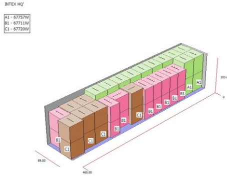
Figure 5. Sample output from the BlackBox, generated via its internal graphics engine. Output can be created in jpg, bmp or pdf format.
